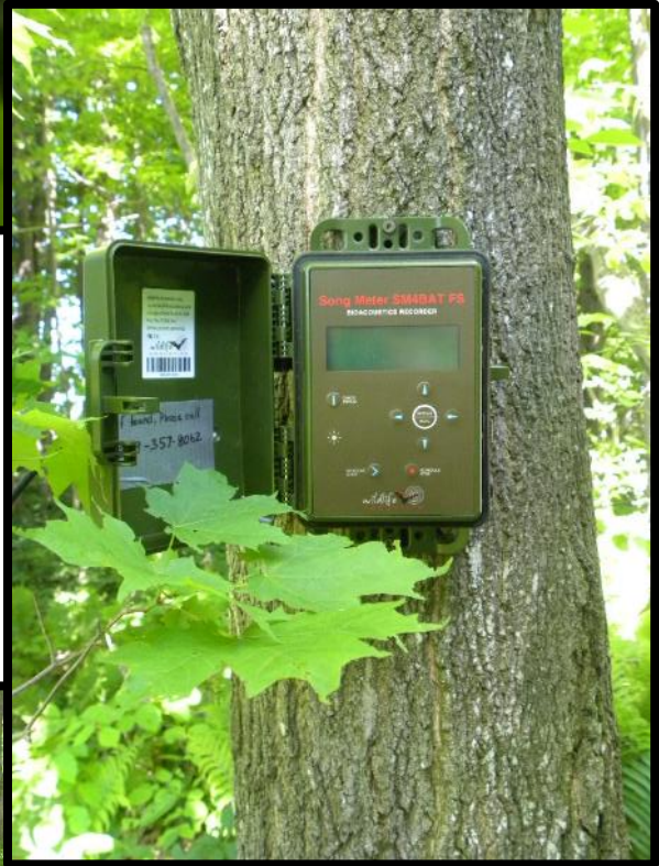
Photo 37: Song Meter SM4BAT FS bioacoustics recorder by Wildlife Acoustics.
