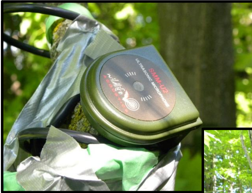
Photo 36: External SMM-U2 ultrasonic microphones attached to the bat meters enhanced the recording distance and clarity.
