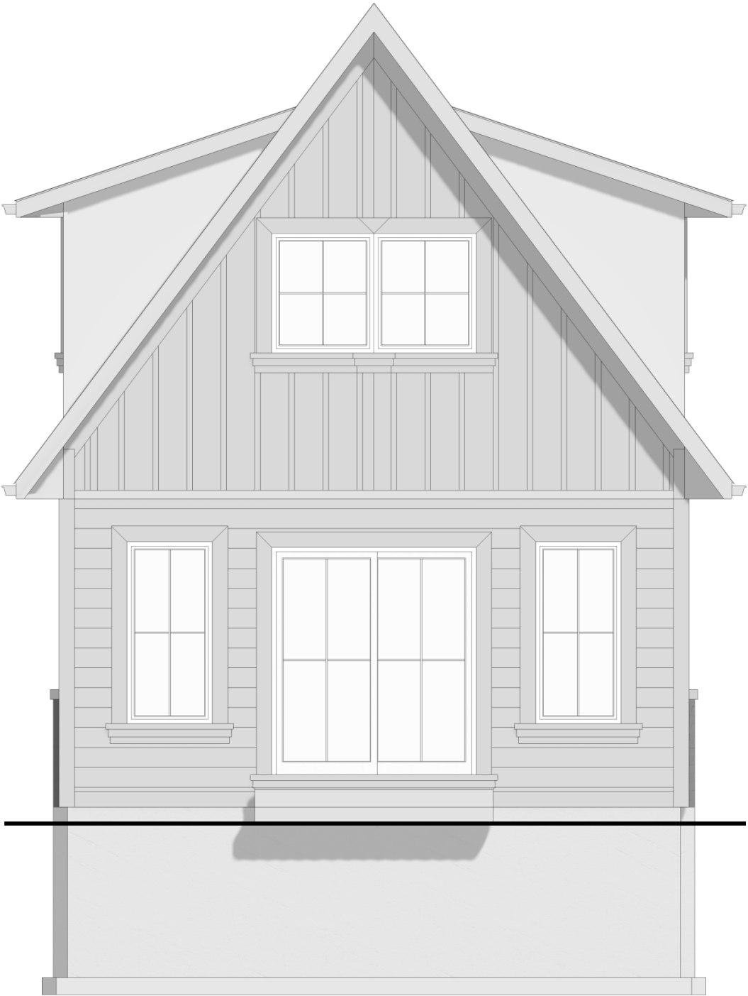
REAR ELEVATION SCALE: 1/4" = 1'-0"
