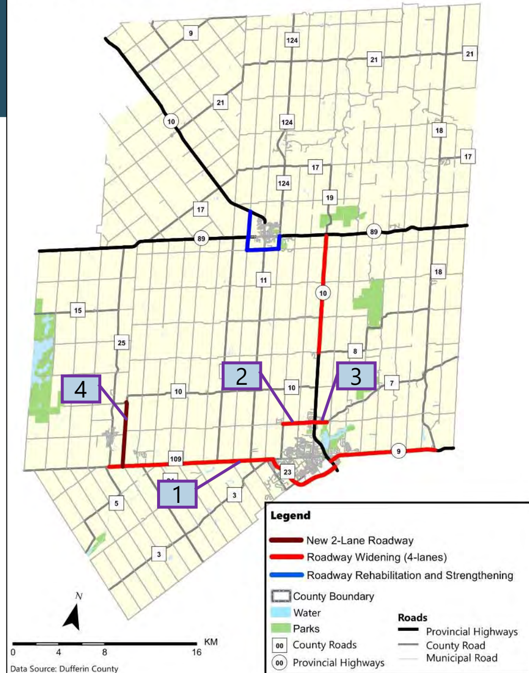
Figure 37. Alternative 3 Roadway Improvements
