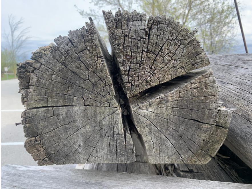
Photo 3: Example of logs splitting
